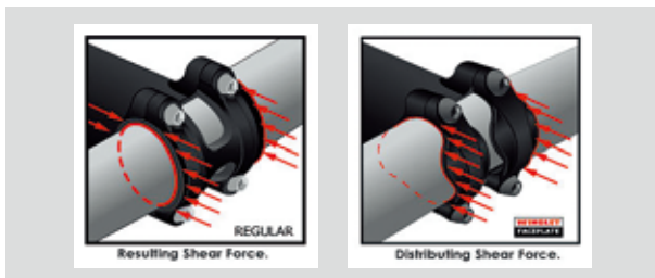
▲ Kalloy's highly original Winglet Faceplate (right) is distinctly different from the conventional design (left).
